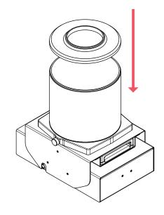
With the correct number of tubes, add the 62mm adapter plate on-top, where the correct filter thread adapter can then be added.
